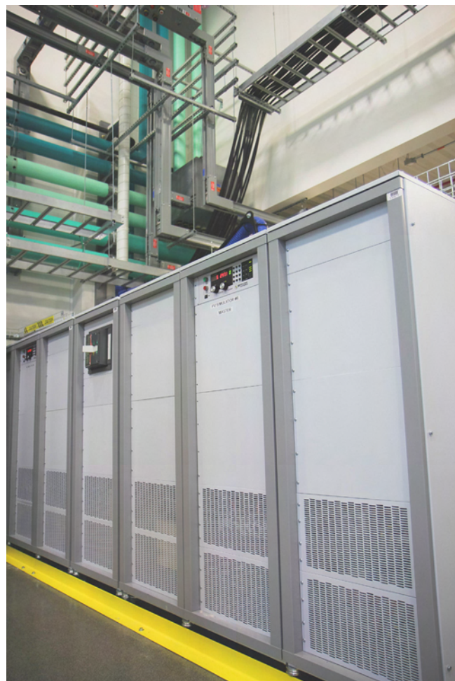
1.5 MW solar array emulator using Magna-Power MT Series power supplies at the National Renewable Energy Laboratory in Golden, CO
