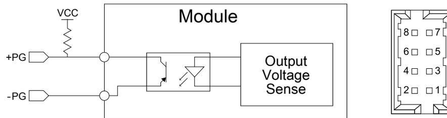
**Figure 5-6.** Dual module *POWER GOOD* wiring diagram
