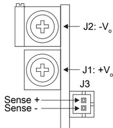
**Figure 6-13.** Bulk module power terminals and sense connector
