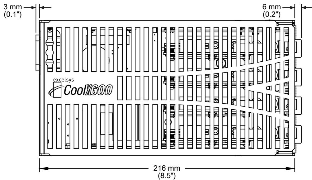
**Figure 6-8.** CoolX IEC version unit dimensions, top view
