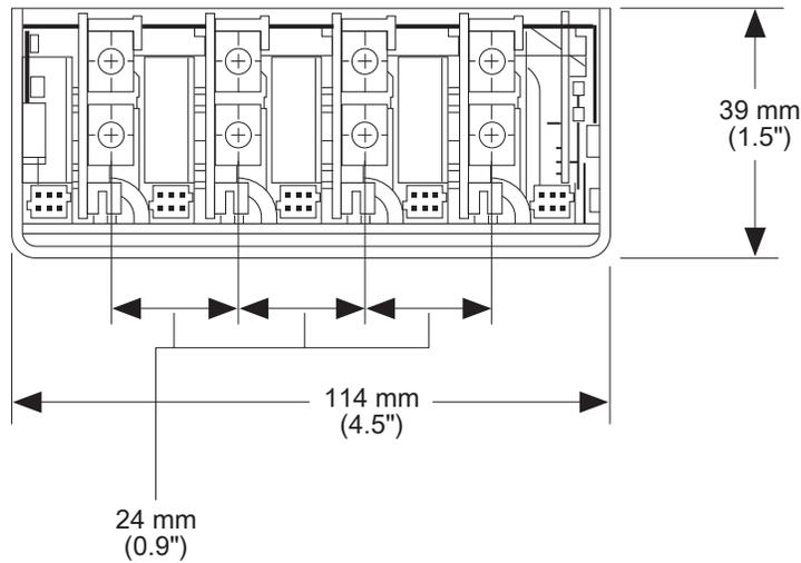
Figure 6-1. CoolX unit dimensions, DC outputs view
