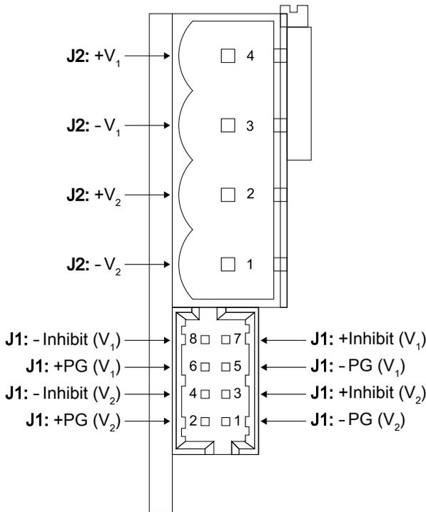
**Figure 6-14.** Dual module power terminals and signal connector
