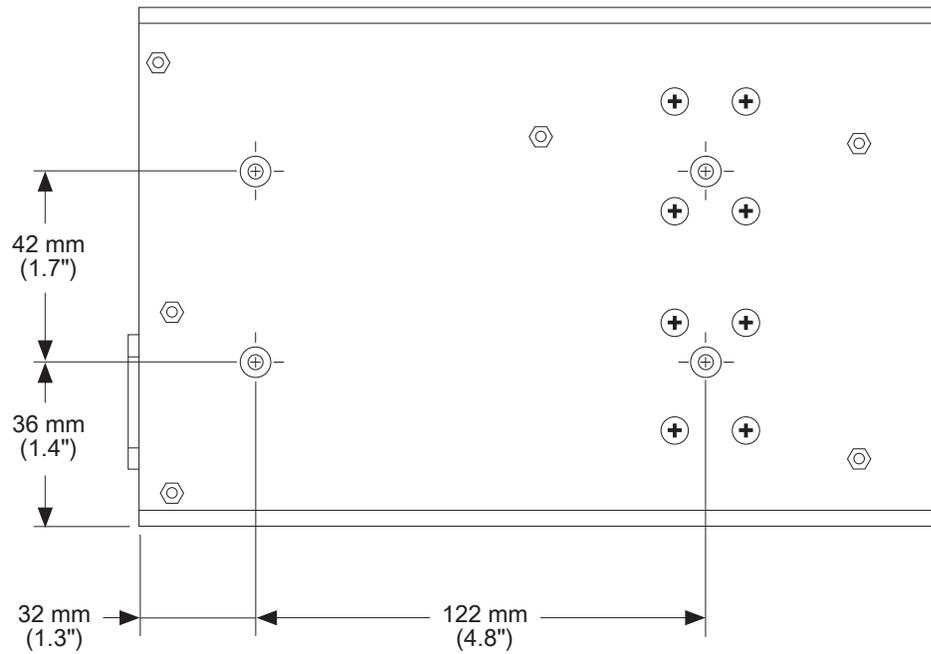
**Figure 6-4.** CoolX unit dimensions, bottom view
