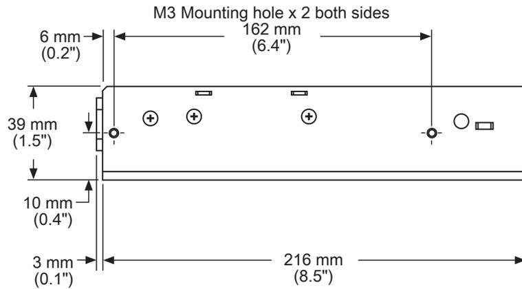
**Figure 6-6.** CoolX IEC version unit dimensions, side view
