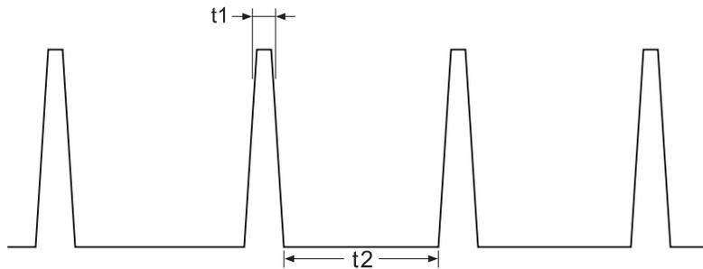
**Figure 3-2. Module hiccup characteristics****Table 3-8. Standard module hiccup characteristics specifications**
