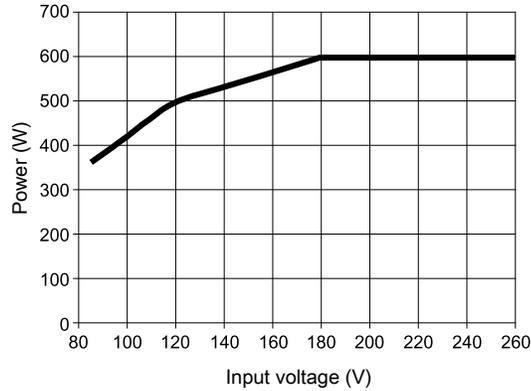
**Figure 6-18.** Chassis line derating
