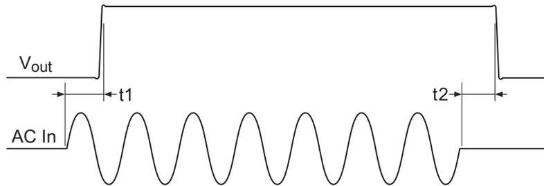
**Figure 3-4.** Module startup/shutdown timing**Table 3-10.** Standard module startup/shutdown timing specifications
