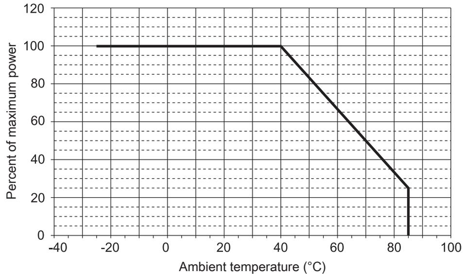
**Figure 6-19.** Chassis and module temperature derating
