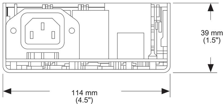
Figure 6-3. CoolX unit dimensions, AC input view
