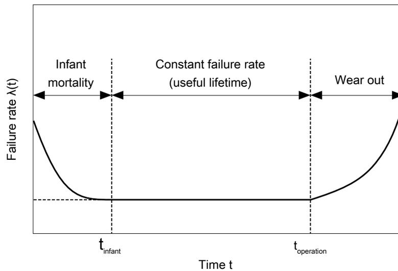
**Figure 6-31.** Failure rate of a power supply
