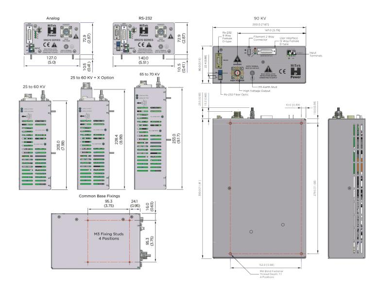
Drawing dimensions are in mm (inches). HV output cable available upon request.
