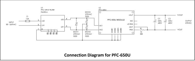
up capacitor up to the peak of the line. After that, internal circuitry will both bypass the external resistor with essentially a short circuit and limit additional inrush current.
