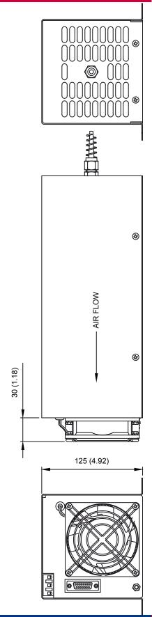
**Drawing dimensions are in mm (inches)** Design developments may result in specification changes
