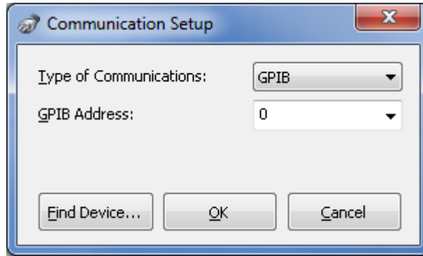
Figure 6.4 GPIB communication setup
