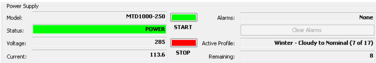
Figure 4.3 Power supply status and control
