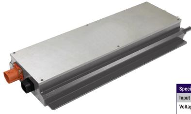
The 3000W LiquaCore® power module is a high voltage liquid cooled DC-DC converter which steps down 400V and provides 12V output, common in hybrid and electric vehicle applications. The output voltage is electrically isolated from the input voltage and suits the conventional 12V accessories and HVAC system requirements of industrial and ecofriendly vehicles.
